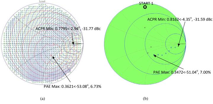
Figure 1: Traditional Load-Pull with 1000 Queries (a) and Sequential Steepest Ascent for PAE (circle) and ACPR (square) with 46 Queries (b)
